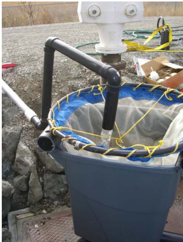
Figure 5-6: Entrainment Sampling Equipment
