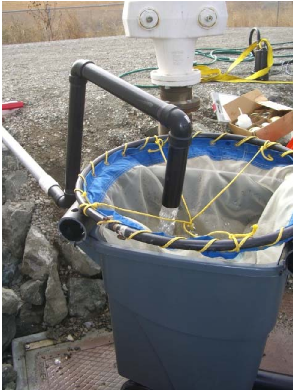
Figure 3-2. Entrainment sampling gear used during the Bay Area Regional Desalination Project pilot plant entrainment study for surveys conducted in November and December 2008.
