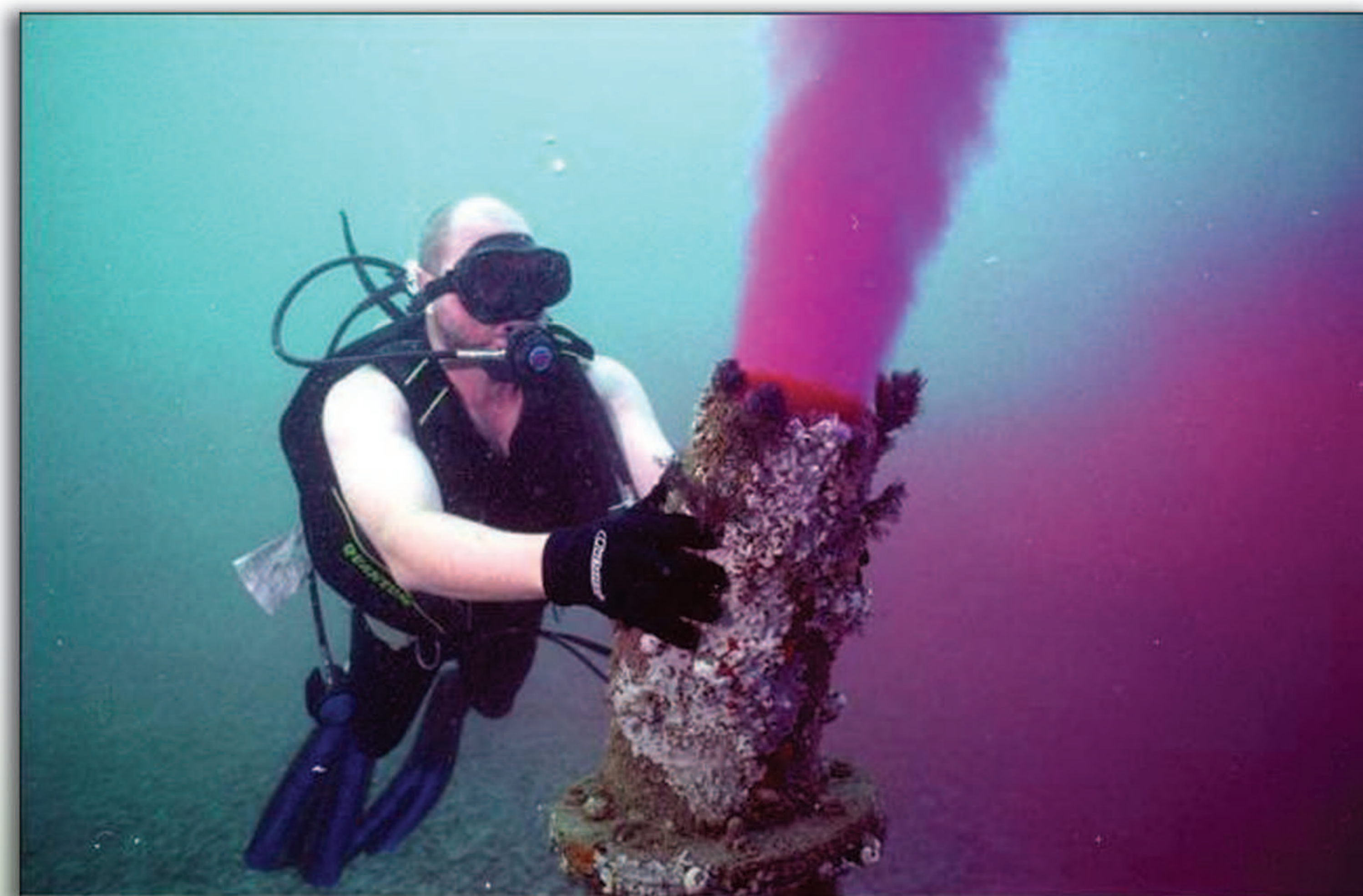
Dye tests being done on the Brine Discharge Ports
